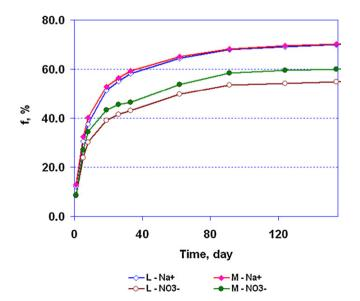
**Fig. 5.** Cumulative leached fractions of Na $^+$  and NO $_3^-$  measured in the laboratory leach test of non-radioactive cementitious wasteform samples subjected (L) and not subjected (M) to  $^{60}$ Co gamma irradiation. The cumulative dose was  $10^6$  Gy.
