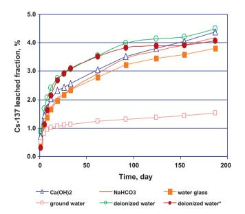
**Fig. 4.** Time-dependent variations in  $^{137}$ Cs cumulative leached fractions f (%) =  $\phi$  100% for the laboratory leach tests of cementitious wasteform samples containing simulated NaNO<sub>3</sub>-rich radioactive waste performed in various leach solution media.
