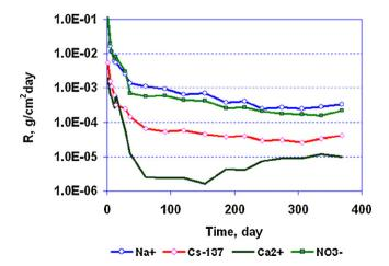
**Fig. 3.** Average normalised leach rates (in this figure R = NR) of  $^{137}Cs^+$ ,  $Na^+$ ,  $Ca^{2+}$  and  $NO_3^-$  from cementitious wasteform samples containing simulated operational radioactive waste rich in NaNO<sub>3</sub> as a function of time.
