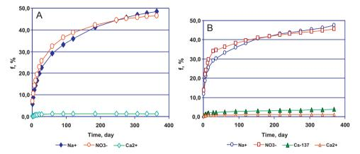
**Fig. 2.** Time-dependent variations in cumulative leached fractions of ion species f(%) for the laboratory leach tests of non-radioactive (A) and radioactive (B) cementitious wasteform samples containing simulated NaNO<sub>3</sub>-rich waste.
